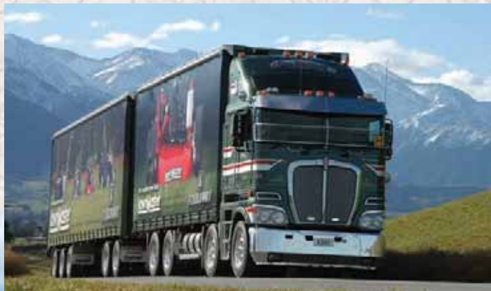
Kenworth K108 truck and trailer on highway with nine axle sets and an extended 23 metre overall length.
