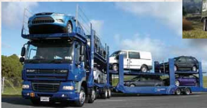
DAF CF85 car transporter – extended length but light overall weight.
