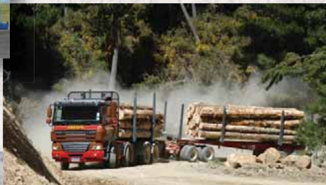
DAF CF85 log truck with extended length to improve stability and safety.
