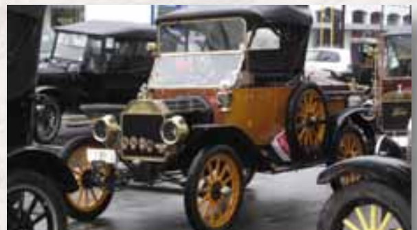
Not all Model T's were black - until 1915 they even had brass radiators.
